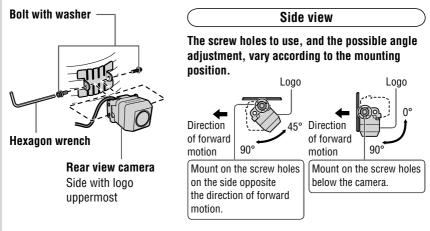
Adjust the camera angle so that the fender or the rear edge of the vehicle appears at the bottom of the monitor.
